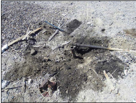
Photograph 29: Suspected former fuel pump and UST location adjacent to SB-3.
