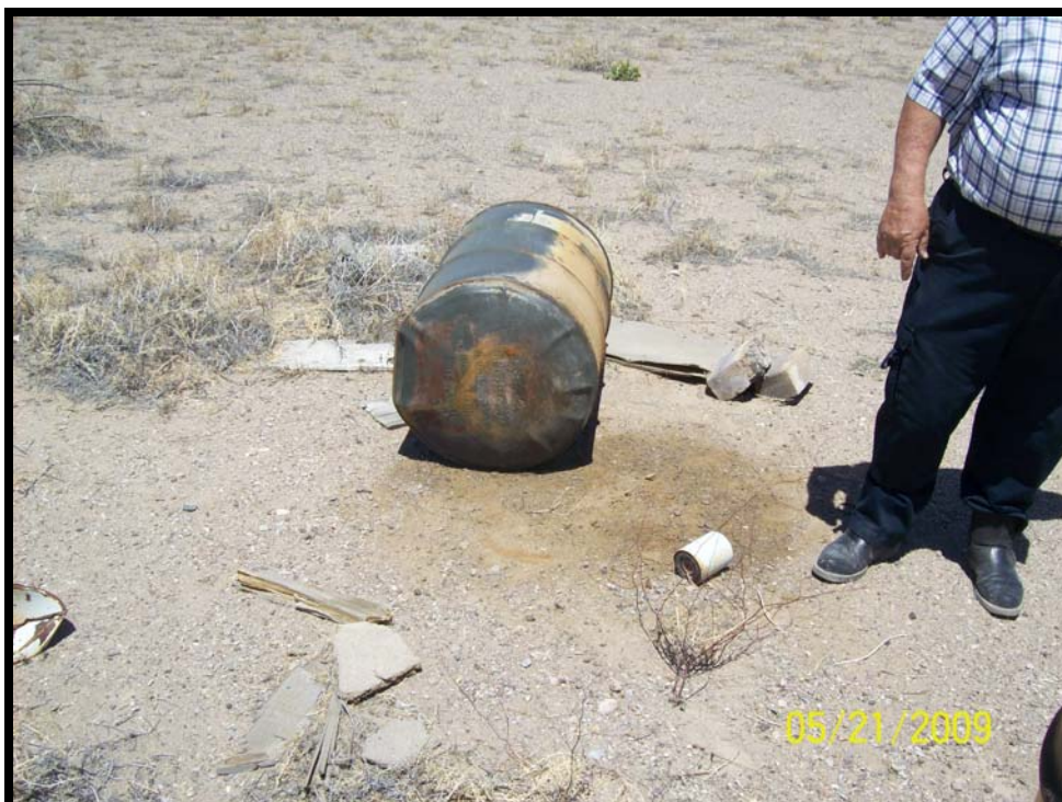
Photograph 10: View of empty 55-gallon drum, oil filter, and stained soil west of hangar.
