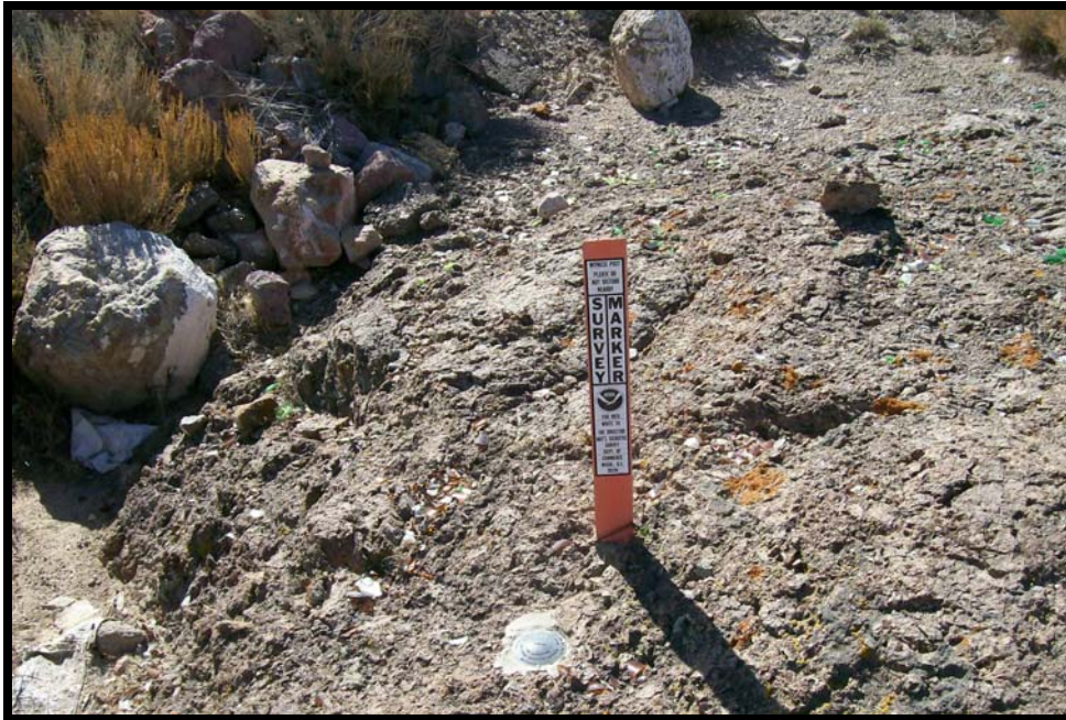
Photograph 13: View of vertical control mark near southeast margin of subject site.
