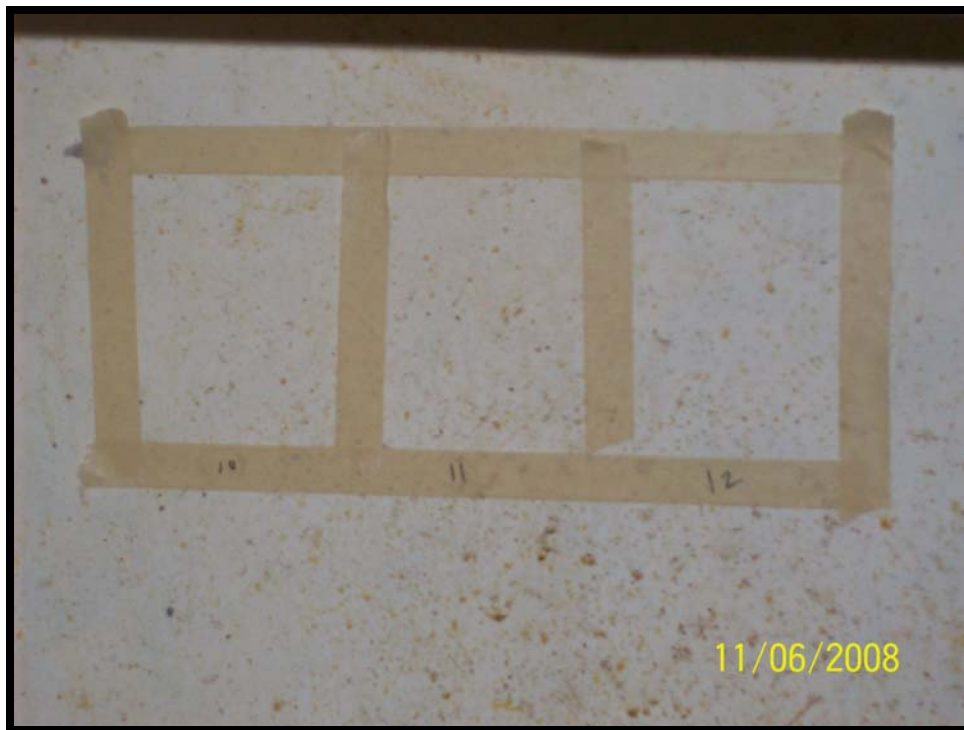
Photograph 5: View of surface wipe sample locations KTN1-SWP-10M, KTN1-SWP-11I, and KTN1-SWP-12L in kitchen.
