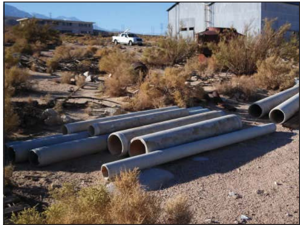
Picture 12—Transite pipe adjacent to the collapsed building.
