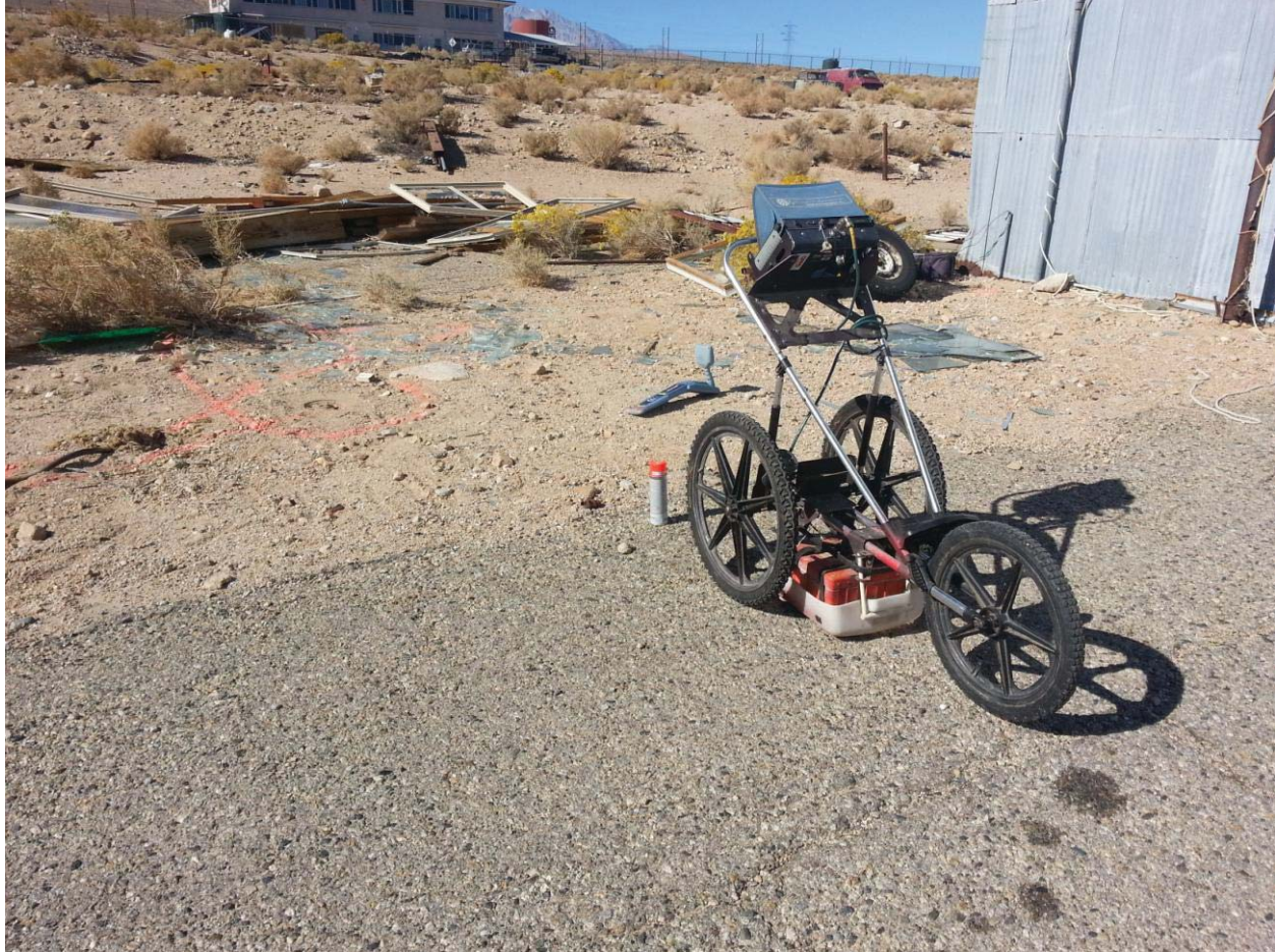
The above photo shows the GPR equipment that was used at the site.
