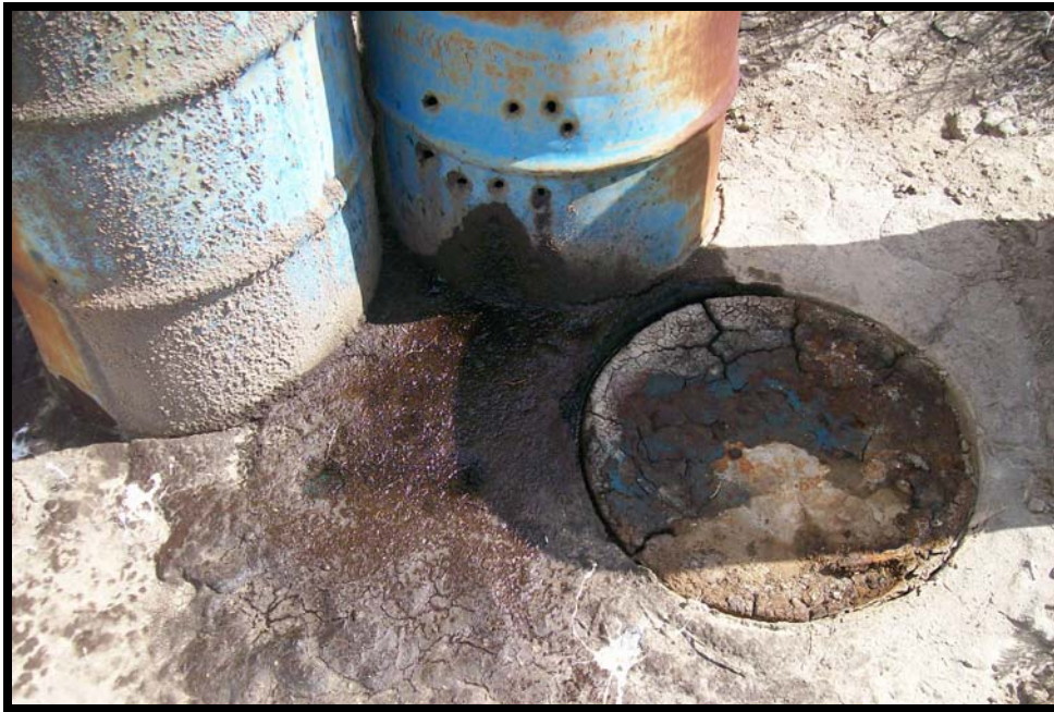
Photograph 15: View of soil staining at base of punctured 55-gallon drums.
